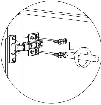
Assemble these four holes first, adjust the door and ensure it is level, then tighten all screws.
